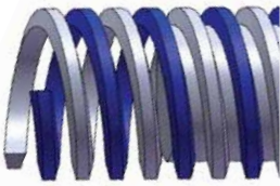
Double Start Screw - Lead is 2 X Pitch
